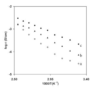
Variation of log  $\sigma$  with reciprocal temperature for (a) PVdF-HFP + DMOImPF<sub>6</sub> + NH<sub>4</sub>PF<sub>6</sub>, (b) PVdF-HFP + DMOImPF<sub>6</sub> + NH<sub>4</sub>PF<sub>6</sub> + DMA and (c) PVdF-HFP + DMOImPF<sub>6</sub> + NH<sub>4</sub>PF<sub>6</sub> + PC.
