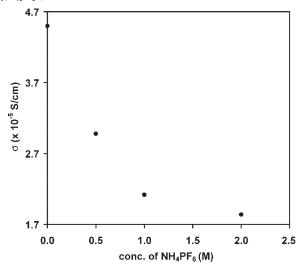
Figure 2. Variation of conductivity of PVdF-HFP + DMOImPF $_6$  + x(M) NH $_4$ PF $_6$  at 30  $^{\circ}$ C with the concentration of salt.
