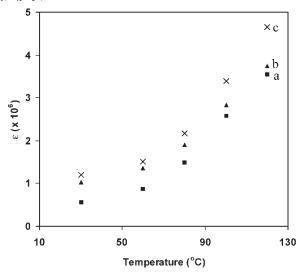
**Figure 4.** Variation of dielectric constant with temperature for (a) PVdF-HFP + DMOImPF<sub>6</sub> + NH<sub>4</sub>PF<sub>6</sub>, (b) PVdF-HFP + DMOImPF<sub>6</sub> + NH<sub>4</sub>PF<sub>6</sub> + 0.1 ml DMA and (c) PVdF-HFP + DMOImPF<sub>6</sub> + NH<sub>4</sub>PF<sub>6</sub> + 0.1 ml PC.
